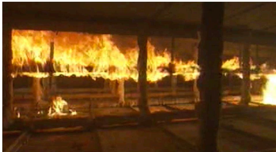
This image, taken from video footage of a test conducted at a nationally recognized test laboratory, shows flame spreading through a plenum space, fueled by cable that is not plenum-rated.
