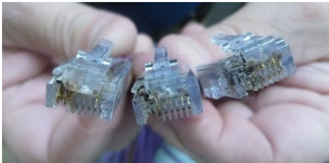
Figure 5: The results of thermal runaway on Pins 7 and 8 caused by a non-compliant RJ45 jack. The use of UL 94V-0 materials allowed the plugs to self-extinguish, whereas materials of a lesser flame rating could have resulted in catastrophic flame spread.
