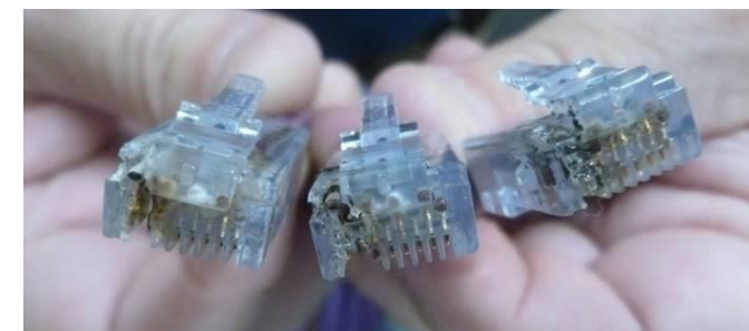
FIGURE 6: RJ45 plug showing the results of thermal runaway on Pins 7 and 8 caused by a non-compliant RJ45 jack. The use of UL 94V-0 materials allowed the plugs to self-extinguish, whereas materials of a lesser flame rating could have resulted in catastrophic flame spread. Source: Sentinel Connector Systems
